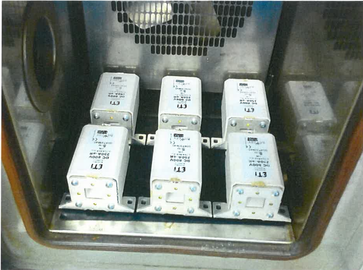
Picture 9: Fuses at the end of warm storage test
