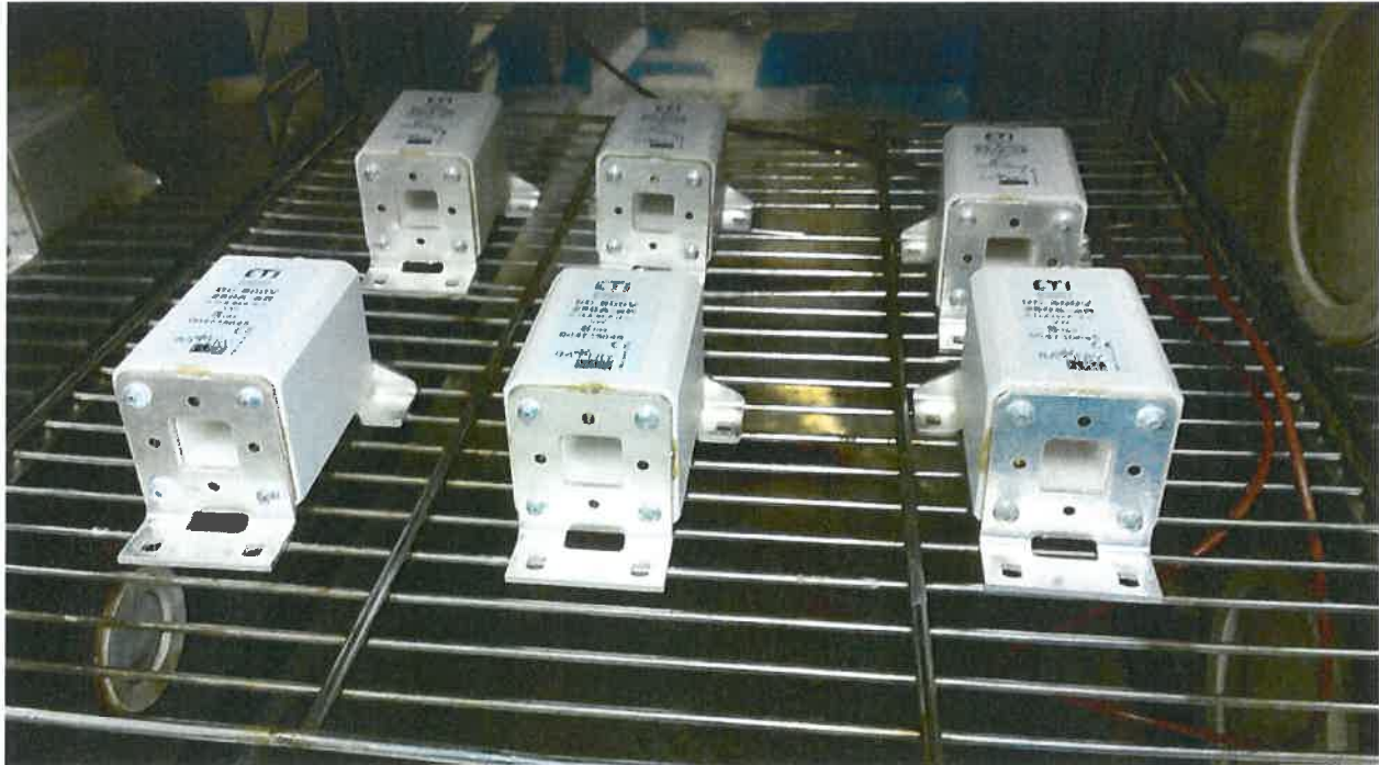
Picture 3: Fuses at the end of temperature cycle test
