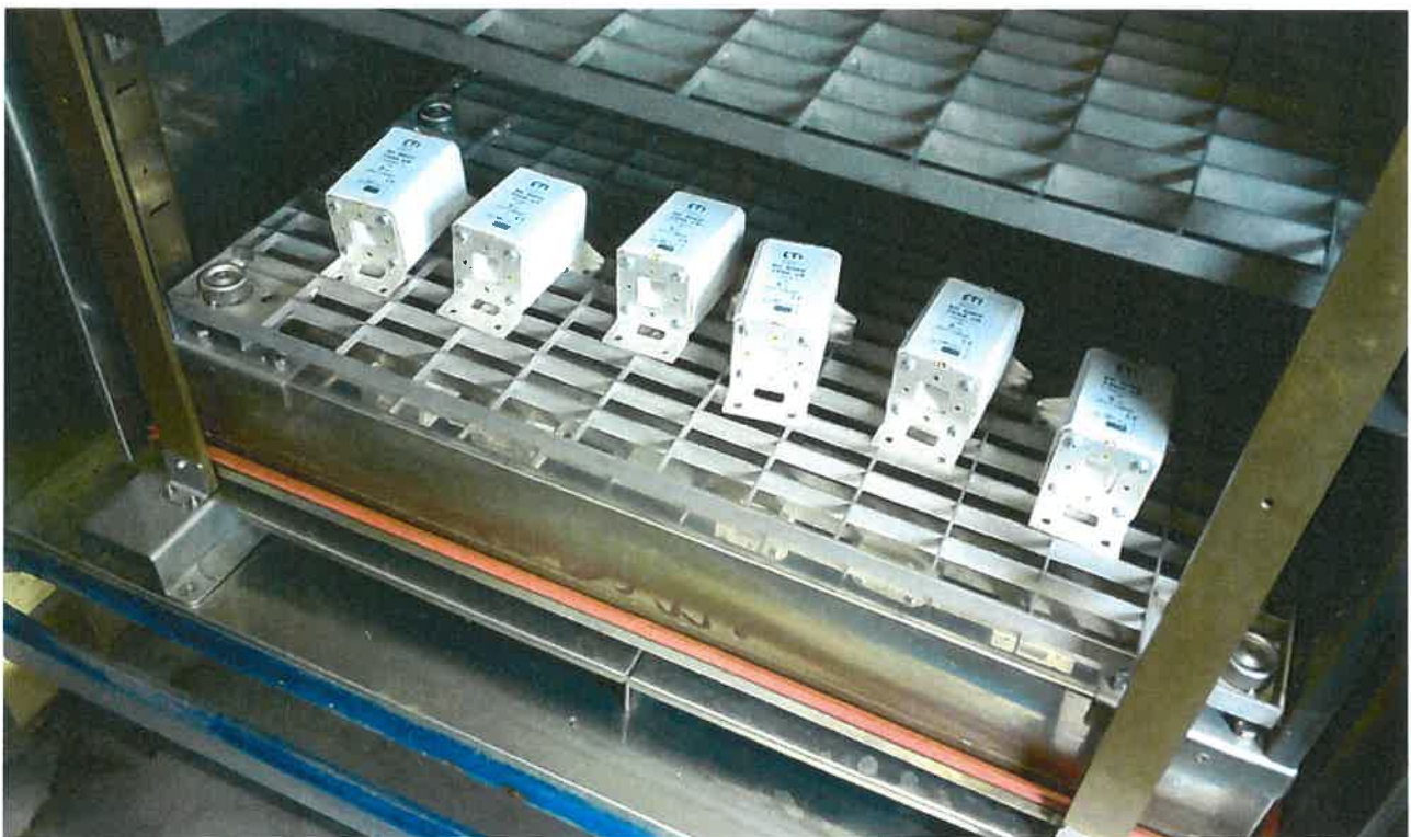
Picture 5: Fuses at the end of thermal shock test
