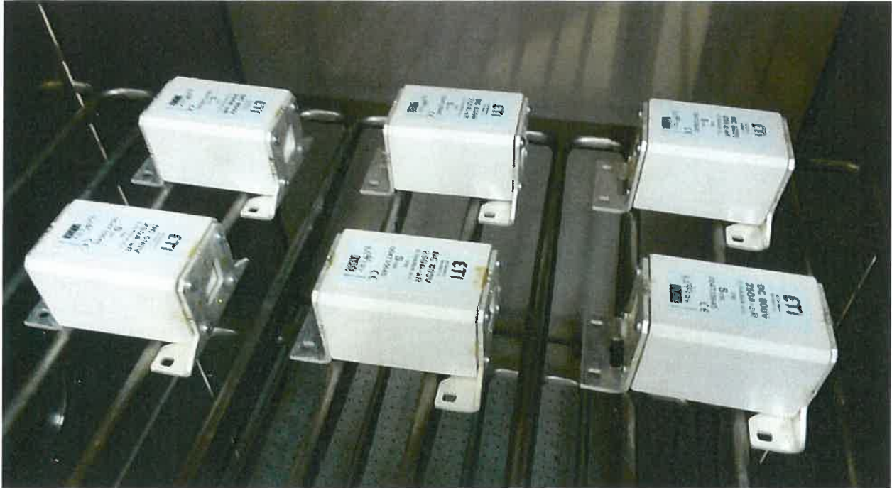
Picture 10: Fuses at the end of cold storage test
