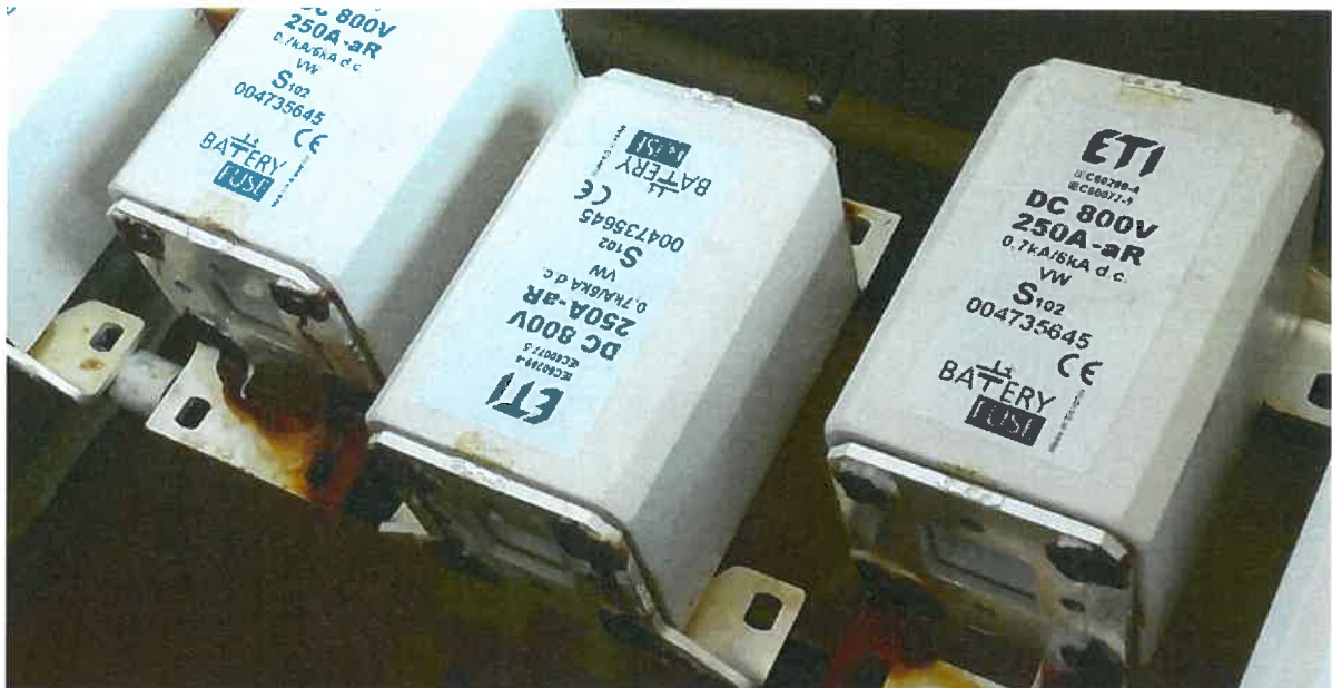
Picture 14: Fuses at the end of salt spray test
