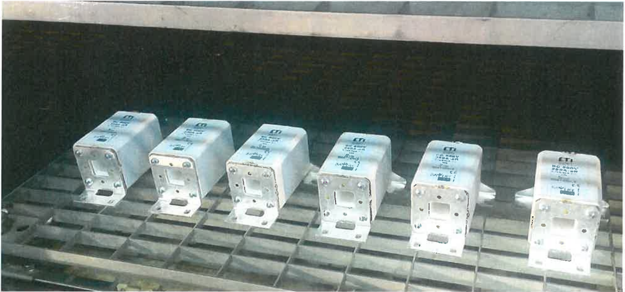
Picture 4: Fuses at the beginning of thermal shock test
