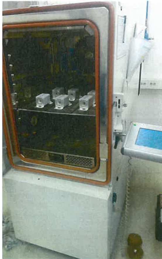
Picture 2: Fuses at the end of damp heat test 2
