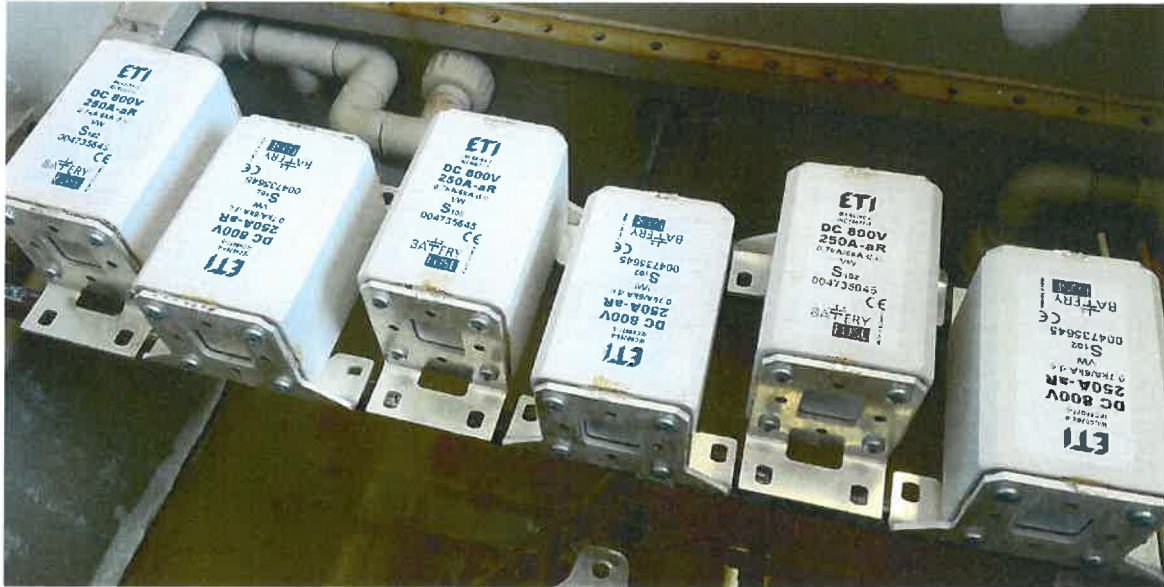
Picture 11: Fuses at the beginning of salt spray test
