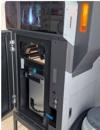
SLS 3D-tiskalnik Formlabs Fuse 1+ 30 W
